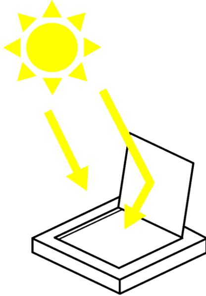
Solar cookers capture solar energy to warm food. They work by reflecting sunlight off the open lid onto the bottom of the box. The bottom is covered with clear plastic wrap to trap the heat. The reflecting surface needs to be angled to direct the maximum amount of sunlight. The box receives sunlight both **directly** from the Sun as well as **reflected** off the lid of the box.
