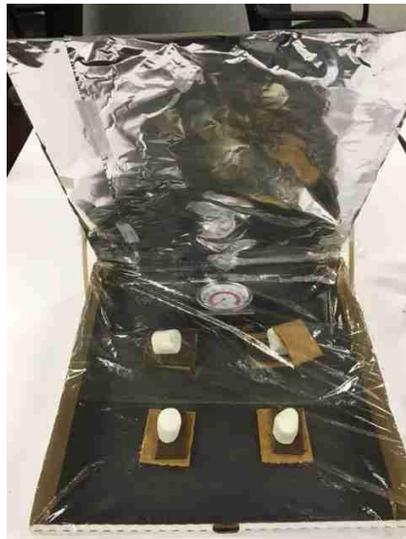
Put your 4 S'mores into the solar cooker. Cover the box opening with plastic wrap. Make sure the box is positioned facing the sun and monitor your S'mores to see if the chocolate and marshmallows are melting.
