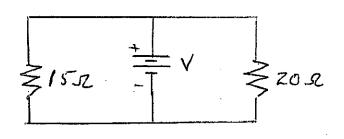
4.4 Find the equivalent resistance for the circuit in Figure P4.4.
