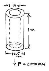
4,56. Referring to Figure 4.33 , let the bar be bored to an inside diameter of 2 cm. Determine the loadings per Example 4.6.
