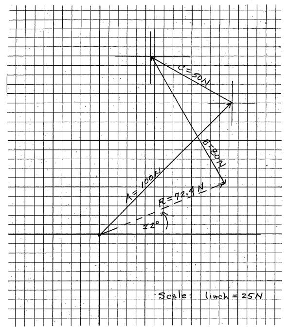
Note: The graphical method requires a large drawing and careful drawing, slight inaccuracies in any vector significantly effect The final result.
