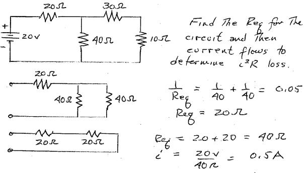
The voltage drop across The ZOR resistance is (V) drop = (0,5 X 20) = 10 V
