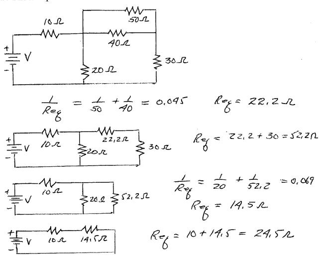
4.5 Find the equivalent resistance for the circuit in Figure P4.5 and the current flow through each resistor.
