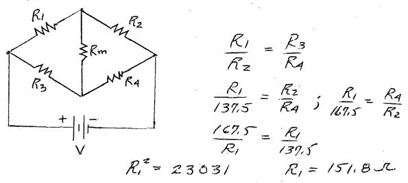
4.28 In a Wheatstone bridge, the resistances  $R_3$  and  $R_4$  are equal. An unknown resistance  $R_1$  is connected to the bridge and the bridge balanced, yielding a value for  $R_2$  of 400 ohms. What is  $R_1$ 's resistance?
