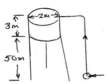
The work is The same = s lifting a full tank 50 m. The mass in The tank is  $m = eV = (1000 \log_{10})(\pi^{2^{2}*3})$  $m = 9424.8 \log_{10}$
