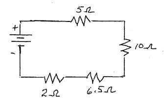
4.2 Find the equivalent resistance for the circuit in Figure P4.2.
