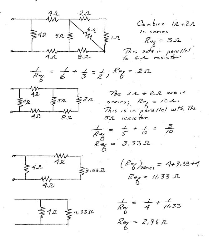
4.12 Find the equivalent resistance for the circuit shown in Figure P4.12.
